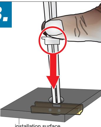
Use the template on the bottom of the page, and secure it to installation surface. Drill hole as shown. Remove after drilling.
