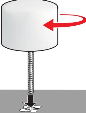
Bend plastic straps until they break off of the flange cap.
